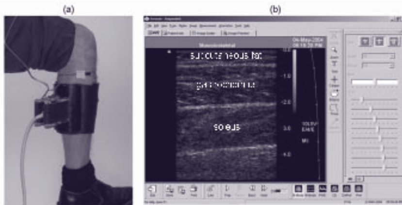
FIGURE 4: (a) Photograph of the ultrasound transducer and strain gauge around the leg. (b) Screen shot taken from the ultrasound scanner showing the muscle anatomy. Notice that the ultrasound scanhead must be held in a stable position during the 10 second periods of data acquisition.
