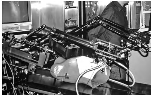
FIGURE 5: Red Dragon is a passive spherical mechanism for precise tracking of forces and torques generated through the surgical instruments along with the tool position during laparoscopic surgery
