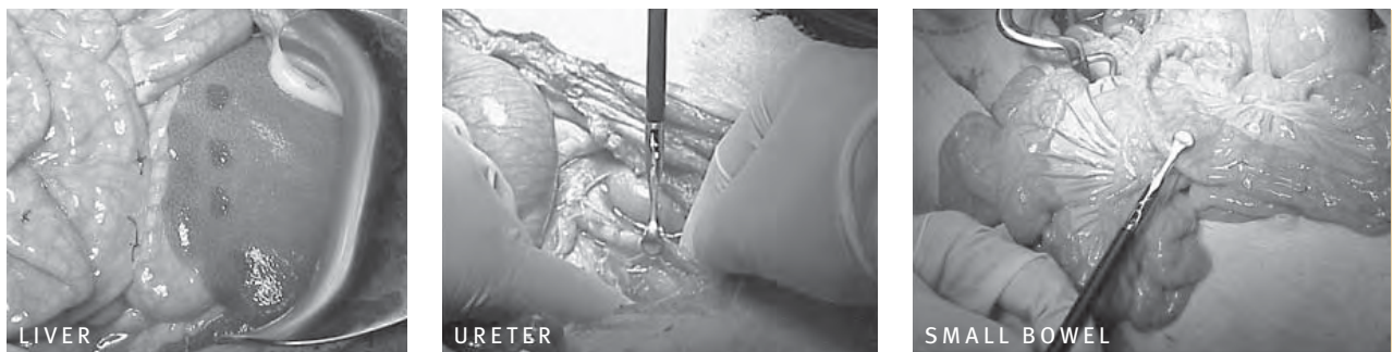
FIGURE 8: Porcine liver, ureter, and small bowel after test grasping with the Motorized Endoscopic Grasper (MEG) for evaluation of the effect of graded stress on tissue integrity and healing.
