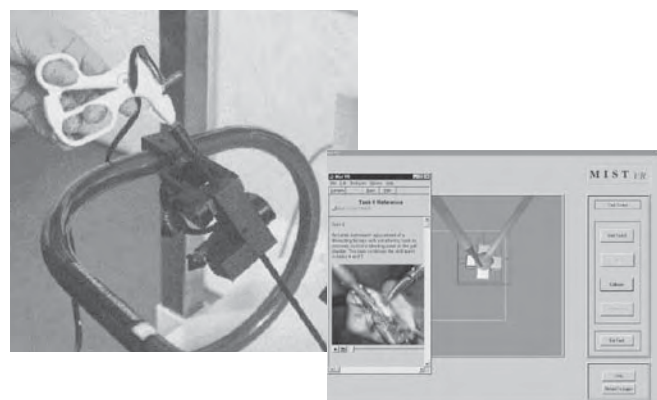
FIGURE 1: MIST-VR basic surgical skills simulator illustrating the image on the simulator screen, and the input handles for tracking motion
