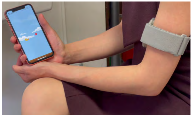
Electromyography (EMG)-driven, smartphone-integrated therapeutic gaming system for rehabilitation.
